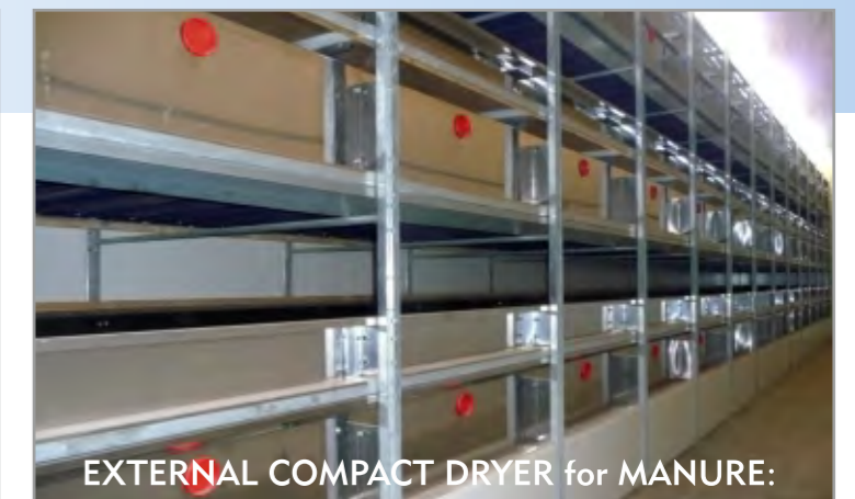
AIR BLOWING with HEAT EXCHANGER
