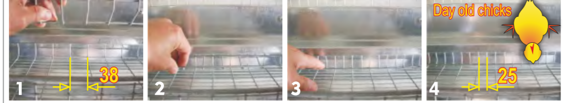
ACCESS TO FEED IS AVAILABLE FROM DAY-OLD TO POINT OF LAY WITHOUT REGULATION. A SIMPLE ADDITIONAL GRILL IS AVAILABLE FOR THE FIRST WEEK. IT REDUCES THE WIRE SPACING FROM 38 TO 25 mm (FROM 1.5" TO 1")
