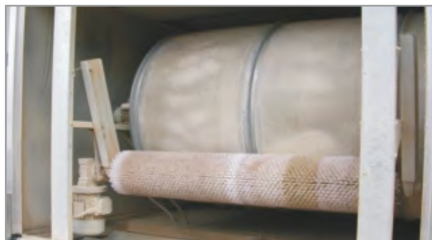
AIR BLOWING MIXING UNIT WITH AUTOMATIC FILTER CLEANING MOD S3 WITH ROTATING BRUSHES SYSTEM
